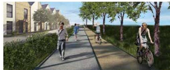
Commuter cycle routes approx 2.5m wide with Commuter route-25m wide cyc segregated footpath total approx width 4.6m
